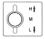
L—LOW SPEED: For hard materials, large drill bit (cutter tools), tapping M—MID SPEED: For the appropriate size, hollow drill, twist drill H—HIGH SPEED: For soft material, small drill bit holder. (cutter tools) L is for low speed, H is for high speed and, M is for medium speed(3 speed models). The drawing is for low speed. Low speed to high speed, turn the knob clockwise, otherwise, anticlockwise.
