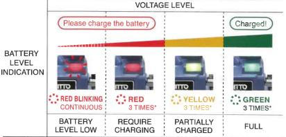
\*After the lamp flashes 3 times with the color according to the battery level, the lamp turns green.
